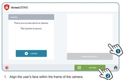
The user's head must turn about 15 degrees right, move to center, and then 15 degrees left. If registered as a User, the system will analyze the face and disarm.
