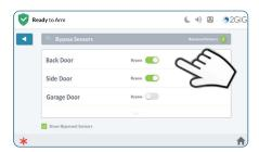
At the Bypassed Sensors screen, tap the switch adjacent to the desired sensor to turn *Bypass* On or Off.
